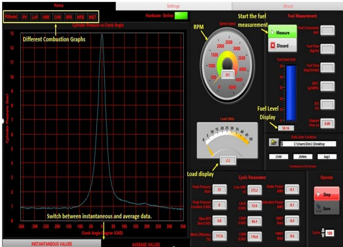
Fig. 3.3.11: EngineScan User Interface- Explained
