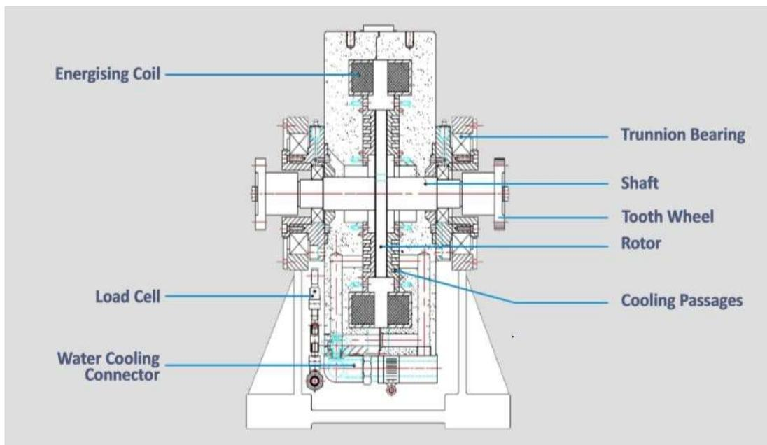
**Fig. 3.2.8: General arrangement of Eddy Current Dynamometer**
