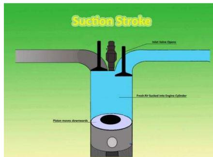
Fig 1. 4. Diesel suction stroke
