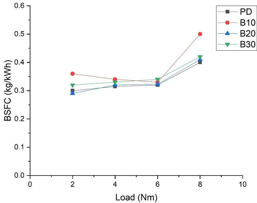
**Fig 5.2 BSFC versus load with various blends.**
