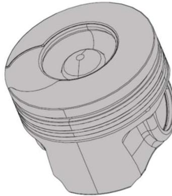
**Fig. 3.2.5: Piston Geometry - Toroidal Combustion Bowl – M&M Jeeto**
