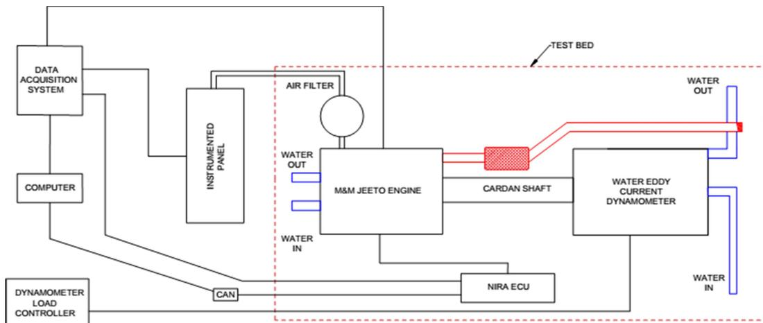
Fig. 3.2: General illustration of engine test setup
