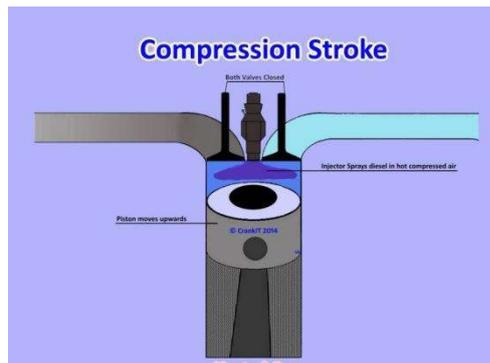
Fig. 1.5 Diesel compression stroke
