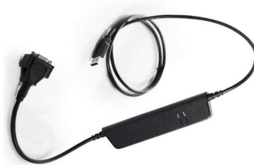
**Fig. 3.2.3: Kvaser Leaf Light V2 CAN Cable**
