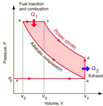
Fig. 1.9 Air standard diesel engine cycle
