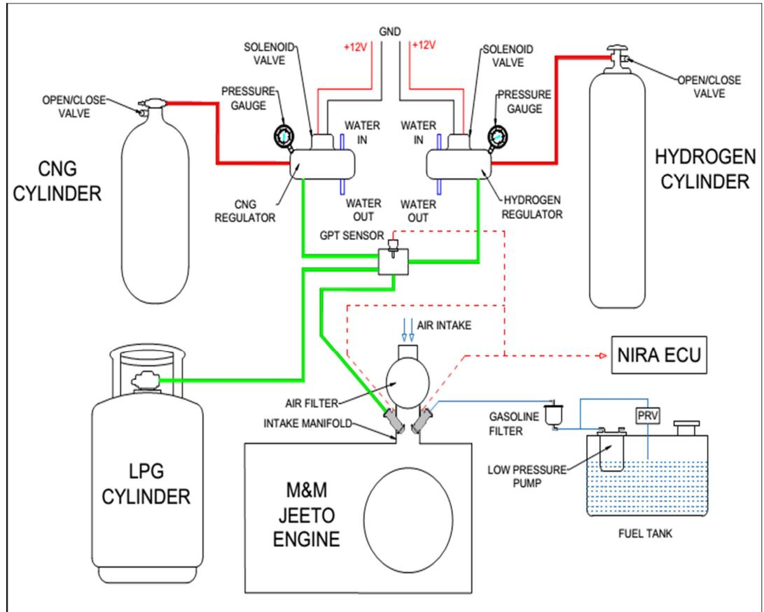
Fig. 3.3: General illustration of diesel secondary fuel injection system.
