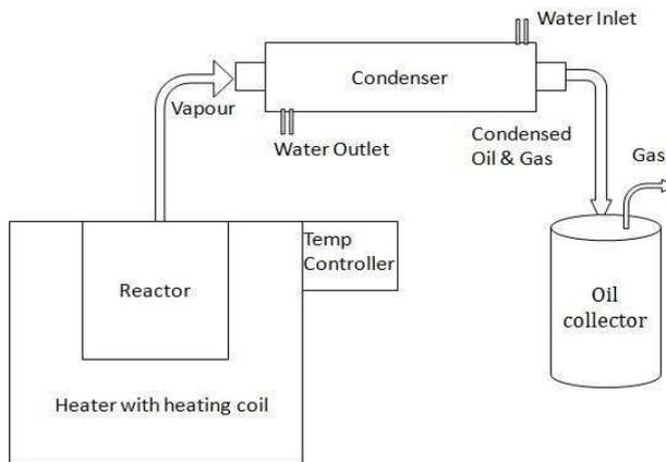
**Figure 4.1 Experimental layout of pyrolysis process**
