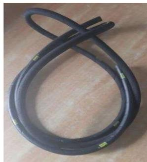
**Fig. 3.4.6: CNG Low Pressure Pipe**
