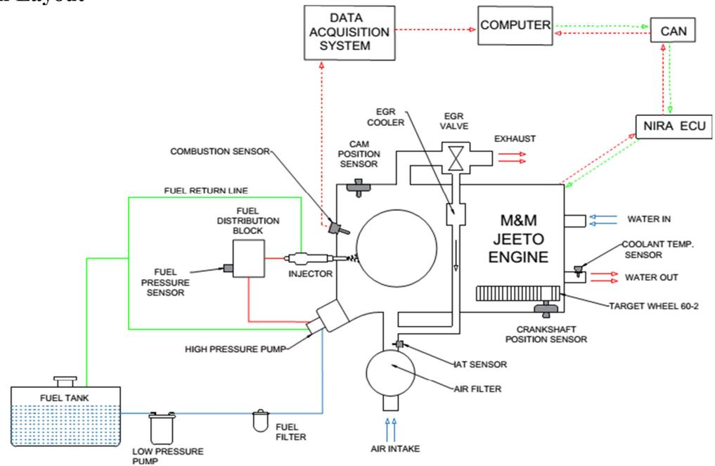
Fig. 3.1.: General illustration of engine fuel system, ECU and data acquisition system
