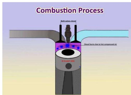
Fig. 1.6 Diesel engine combustion
