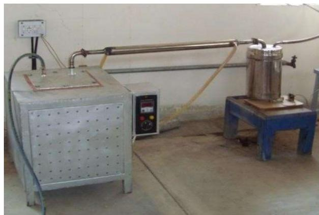
**Figure 4.2 Experimental setup of Pyrolysis process**
