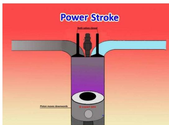
Fig. 1.7 Diesel power stroke
