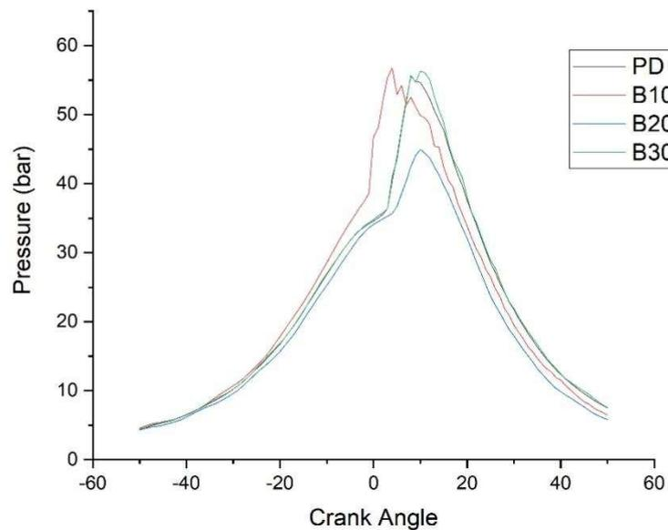
**Fig 5.3 pressure versus crank angle with different blends.**
