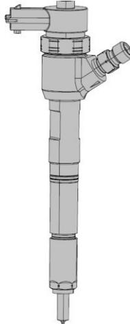
**Fig. 3.2.6: Fuel Injector M&M Jeeto**
