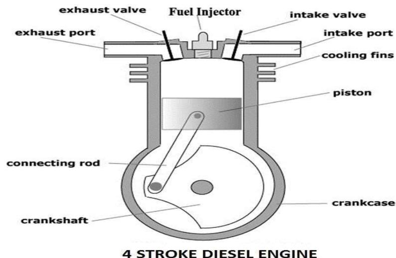
Fig 1.1 4 stroke diesel engine
