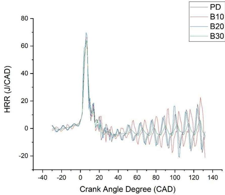
**fig 5.4 HRR versus CRANK angle with different blends**
