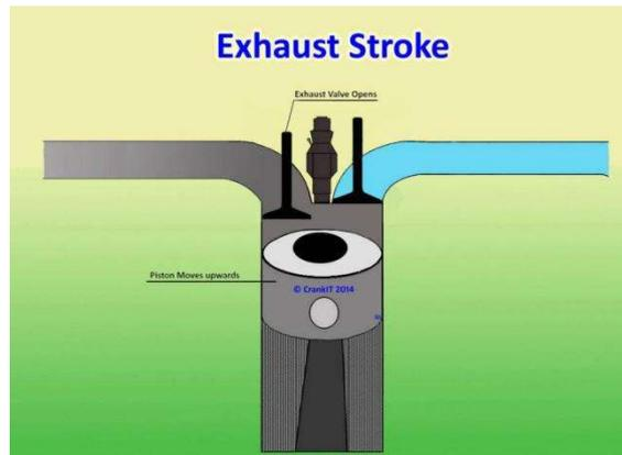
Fig.1.8 Diesel exhaust stroke
