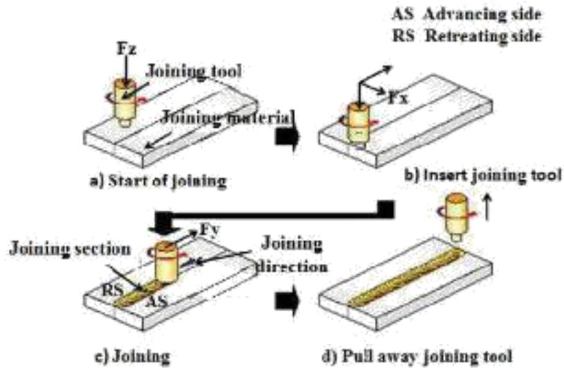
**Fig. 1.1 Schematic representation of FSW [3]**
