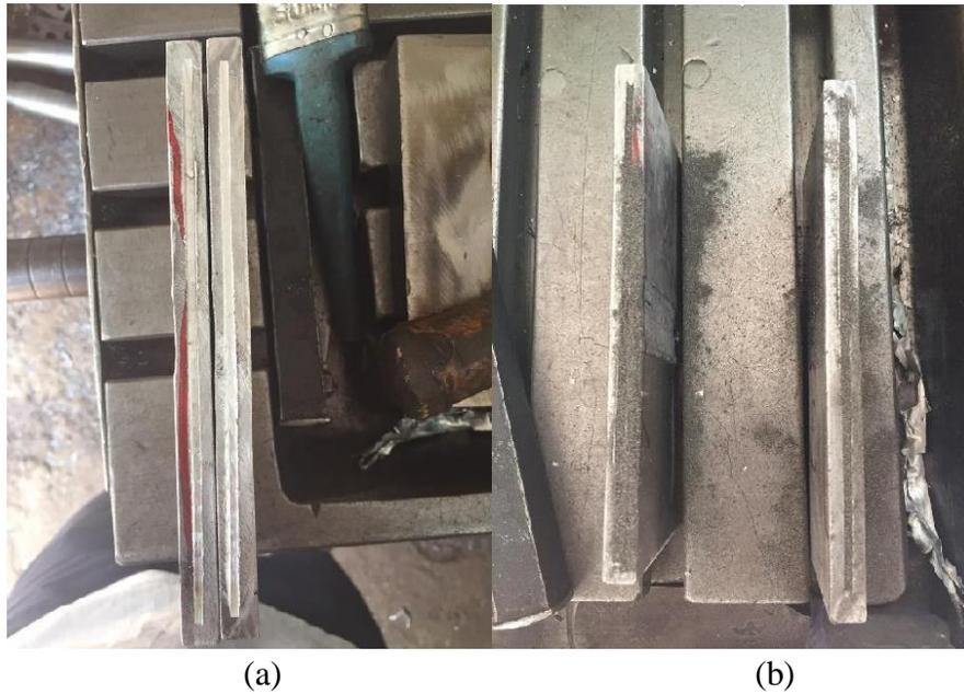
**Figure4.10: image (a) showing the groove made in the plates & image (b) showing the powder filled in the grooves**
