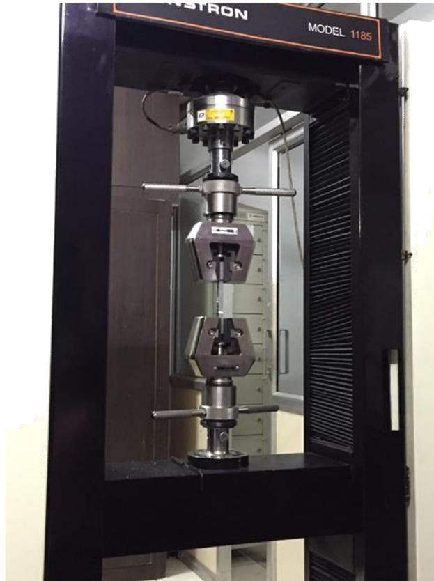
**Figure4.12: specimen mounted over the universal testing machine (instron)**
