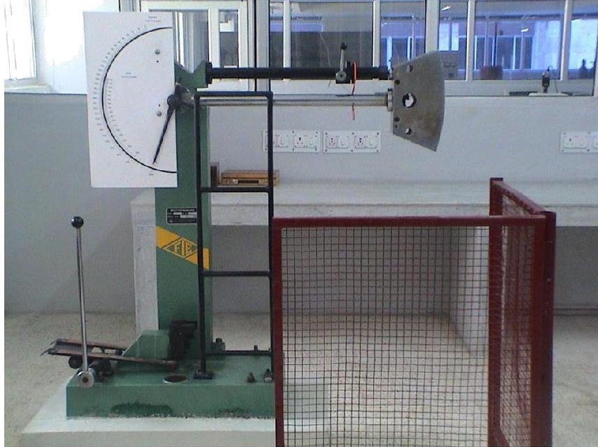
**Figure4.16: image showing impact testing machine**
