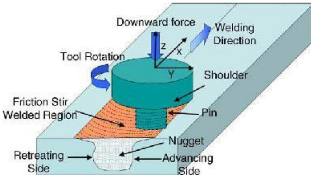
**Fig. 1.2 Friction stir welding [5]**
