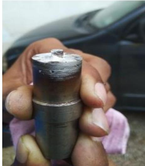
**Figure4.5: Actual image of friction stir welding tool**
