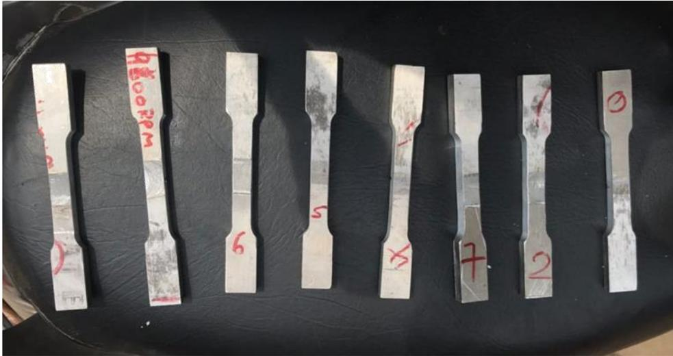
**Figure4.13: image showing the samples for tensile test**
