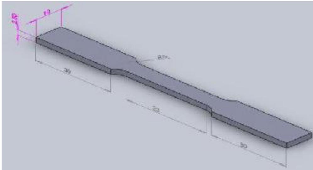
**Fig 4.14: Tensile test specimen with dimensions**
