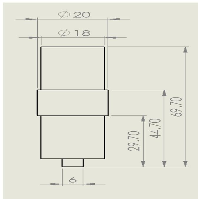
**Fig4.2: 2-d model of designed tool in cad software in front view**
