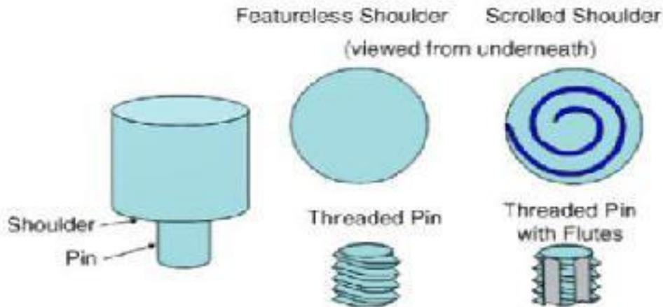
Fig.2.1 Schematic diagram of the FSW tool [5]
