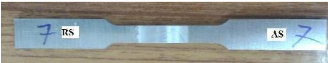
**Fig.5.1 Tensile test specimen for welded material**
