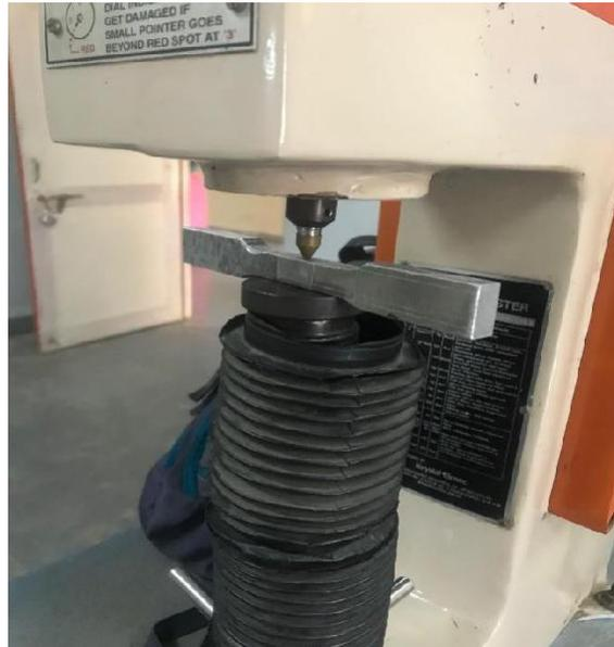
**Figure4.15: image showing hardness testing machine**
