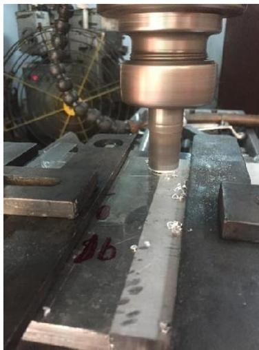
**Figure4.9: AA6061 &AA6351 plates being welded without powder**
