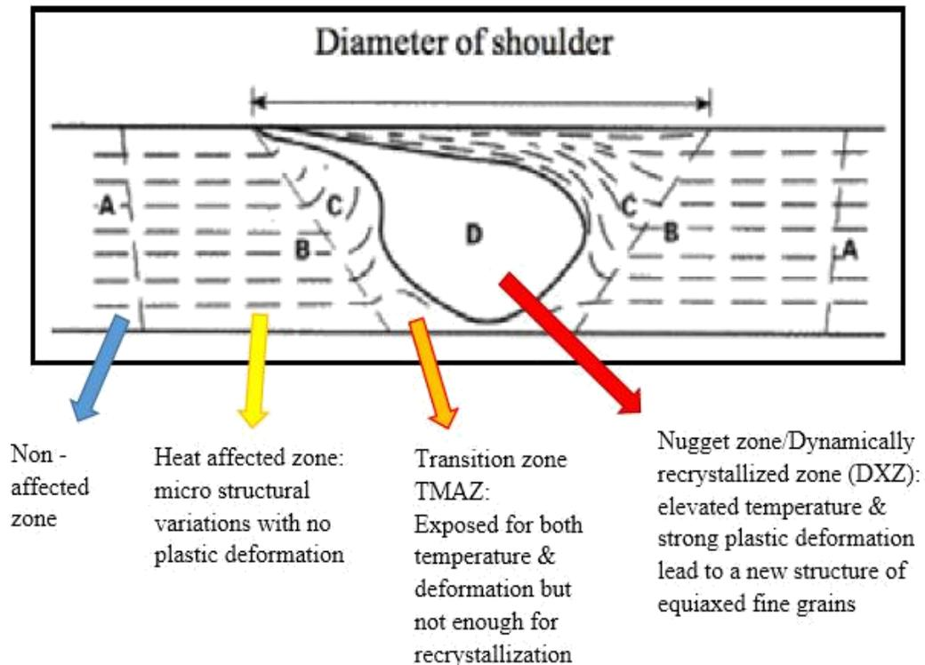
**Fig 2.4: Showing the microstructure zones**
