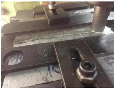
**Figure4.7: Welding plates clamped over fixture**
