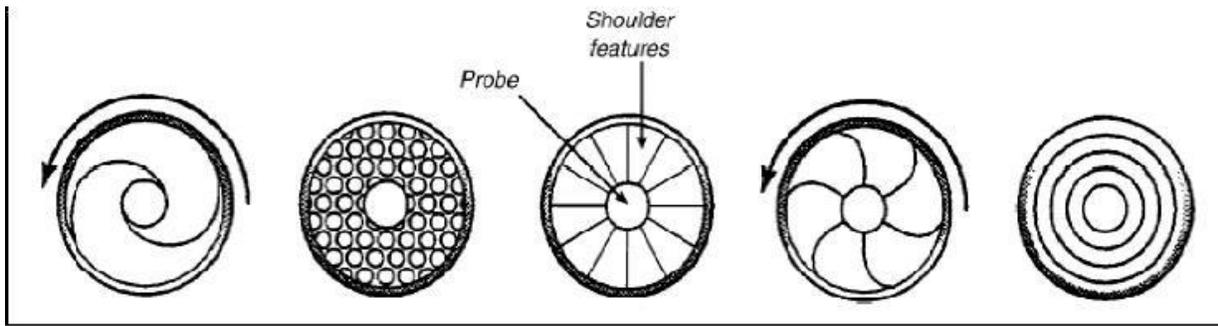
**Fig.2.2 Tool shoulder geometries, viewed from underneath the shoulder [5]**
