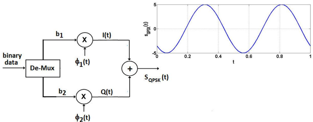
Analyze the Block Diagram given below to obtain the modulation scheme and hence the
