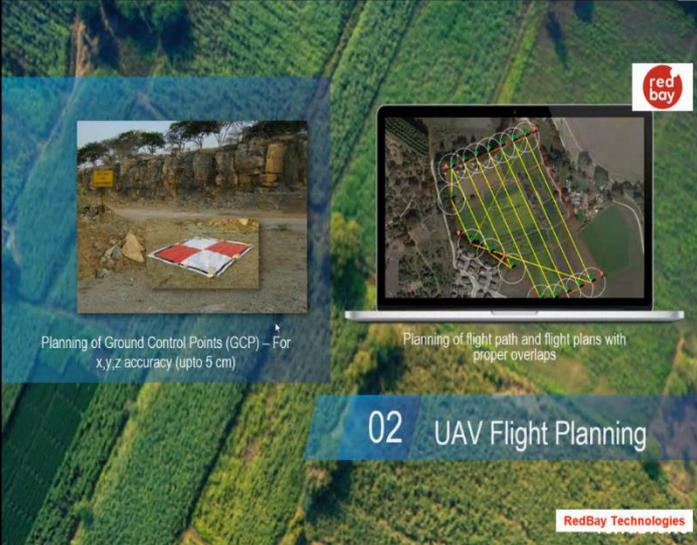
Planning of Ground Control Points (GCP) – For x,y,z accuracy (upto 5 cm)
